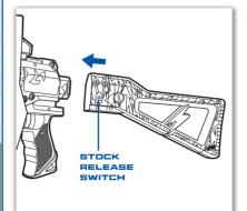
6 Slide STOCK on until it clicks into place. To remove, slide STOCK RELEASE SWITCH down.
